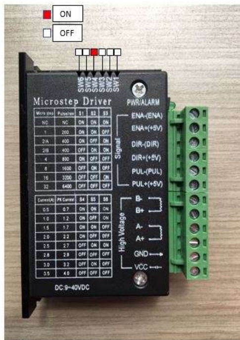
Fig. 1: Diagram of Micro-Step Driver and its connections
